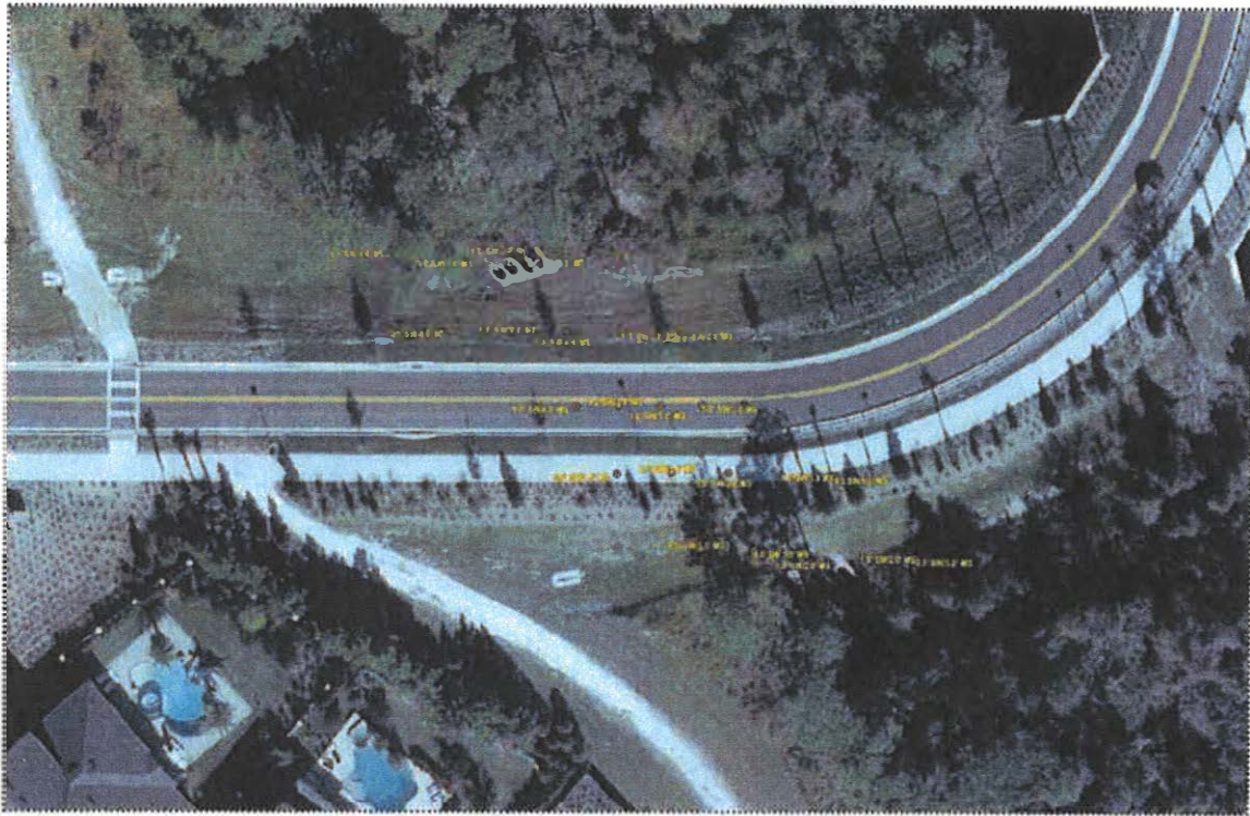
Exhibit 4.1 Muck probe data along Quad 36 note: SW = standing water, MS = mucky sand, S = sand
